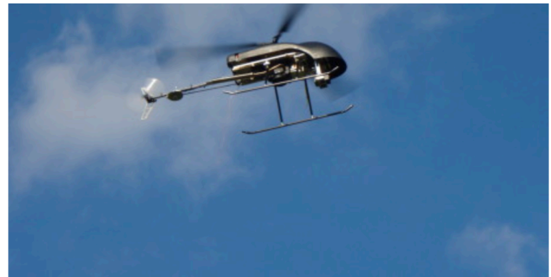
(b) Due to their small size and low weight, IMUs can be used to estimate the orientation for control of an unmanned helicopter.
