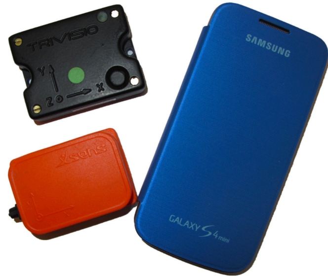
(a) Left bottom: an Xsens MTx IMU [155]. Left top: a Trivisio Colibri Wireless IMU [147]. Right: a Samsung Galaxy S4 mini smartphone.
