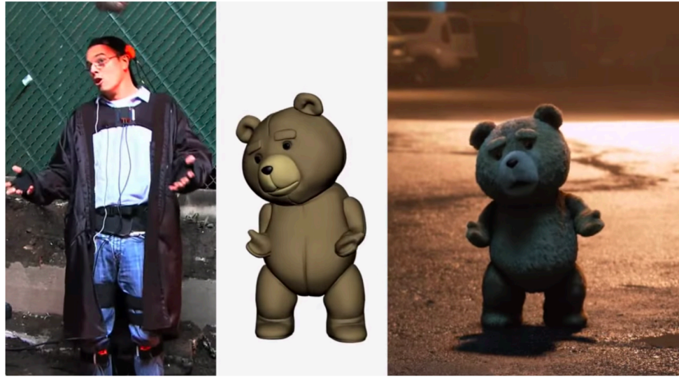
(b) Actor Seth MacFarlane wearing 17 IMUs to capture his motion and animate the bear Ted. The IMUs are placed on different body segments and provide information about the relative position and orientation of each of these segments.
