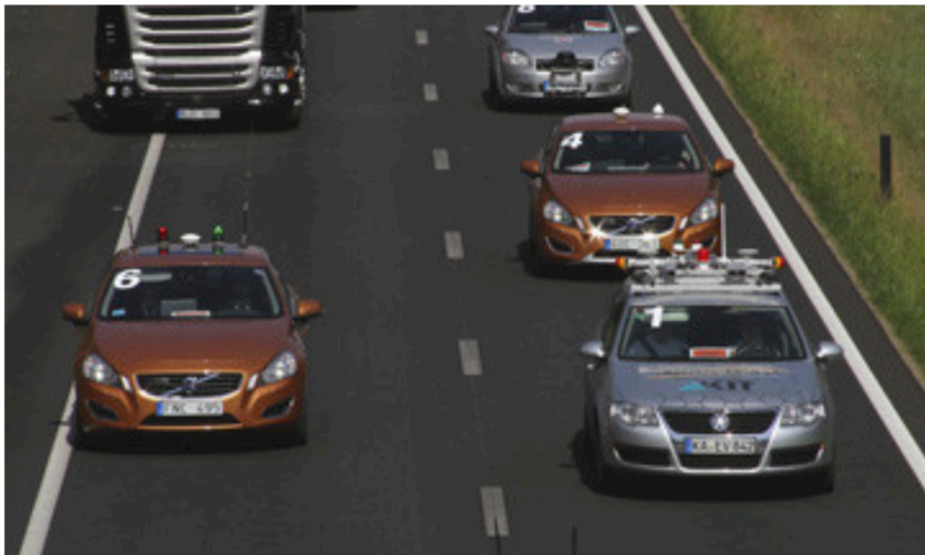
(a) Inertial sensors are used in combination with GNSS measurements to estimate the position of the cars in a challenge on cooperative and autonomous driving.
